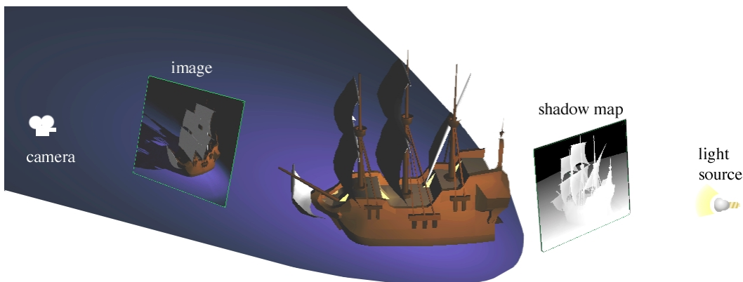
Figure 6.1: Shadow map principle. A shadow map is computed from the point of view of the light source (z-values are represented as grey levels). Then each point in the final image is tested for shadow occlusion by projecting it back in the shadow map (gallion model courtesy of Viewpoint Datalab).
