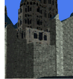
B: Resolution mismatch. Aliasing artifacts occur as the user moves too close to an impostor with a fixed texture resolution.
