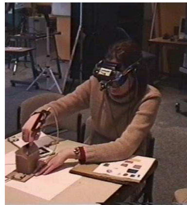
Figure 3: Snapshot of the system in action. Equipped with a tracked HMD, the user interactively paints on a real tracked object.
